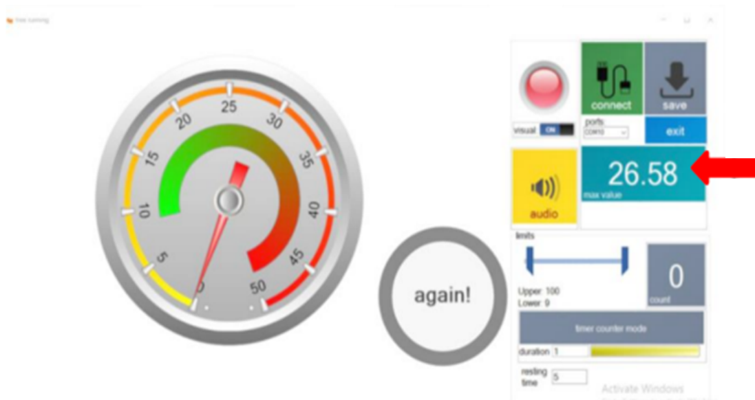
Figure 3. Gauge section display view, max value measured and pointed out
